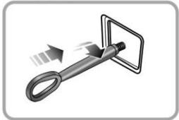
The removable cover is secured to the bumper by a plastic cord. Some models do not have rear towing function. The towing point is intended for use by qualified recovery specialists to assist in the recovery of your vehicle when a breakdown or accident occurs. It is not designed for towing other vehicles. The vehicle can be towed using a tow rope but a towing bar is recommended.
