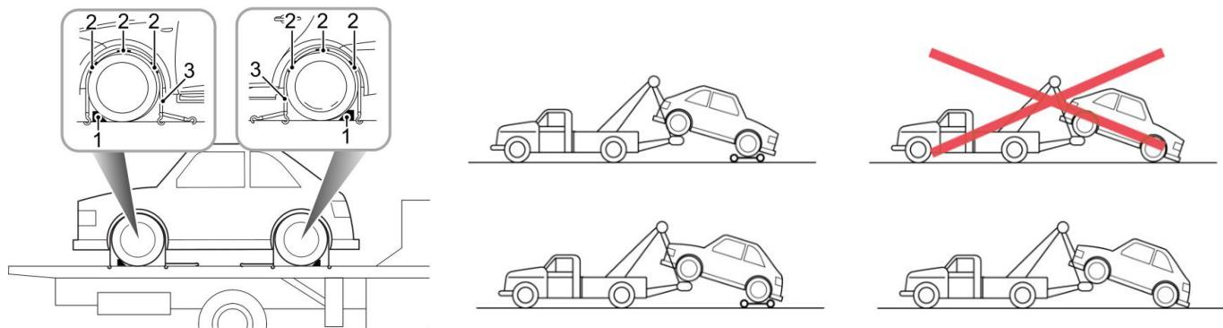
Vehicle Transport & Suspended Towing: Apply the parking brake and ensure the shift control is in P position. See Chapter 2. Immobilisation / Stabilisation / Lifting.
