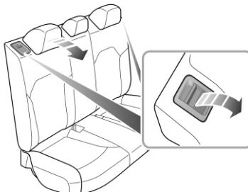
To increase the luggage space, the rear seat backrest can be fully folded forward. When folding the backrest completely, insert the rear seat belt buckles into the corresponding clasps first, then pull the respective control lever at the top of the seat backrest upwards and fold the seat backrest forward.
