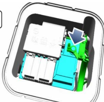
Power off and disconnect the negative cable of 12V low-voltage battery.
